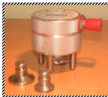
PAT testing head model 6.3kN
